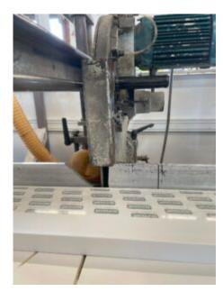
The Health and Safety Executive (HSE) investigation found that the company had not conducted a suitable and sufficient risk assessment of the cross-cut saw, failed to identify the need to adjust the nose guard of the saw to minimise the amount of blade exposed, and failed to identify the need to dry the materials before cutting.
