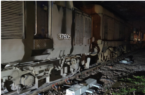
The derailed locomotive
