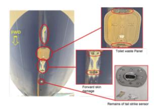
The aircraft was approaching Runway 27L at London Heathrow Airport at the end of a flight from Dubai. During the flare for landing the aircraft "floated" and the crew believed it would not land within the runway Touchdown Zone (TDZ). A go-around was initiated from low height and speed; the subsequent pitch rate caused the aircraft to reach a nose-up attitude sufficient to cause a tailstrike. The aircraft subsequently landed safely and there were no injuries to crew or passengers.
