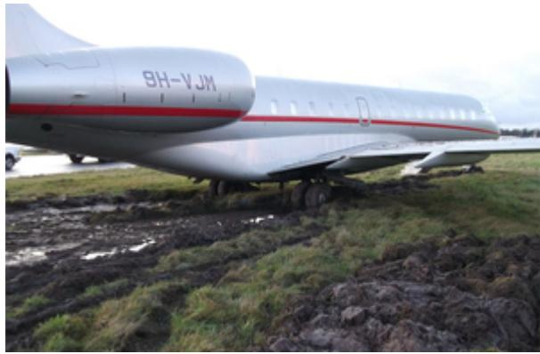
The aircraft, a Bombardier BD-700-1A10 Global 6000 (9H-VJM), suffered a nosewheel steering failure shortly after touchdown. During the subsequent landing roll, directional control was lost due to the inadvertent application of right braking and the aircraft departed the runway surface onto the grass.
