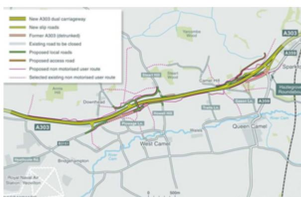
The Order grants development consent for a continuous dual carriageway on the A303 linking the Podimore Roundabout and the Sparkford Bypass. The Proposed Development would also involve the removal of at-grade junctions and direct accesses.
