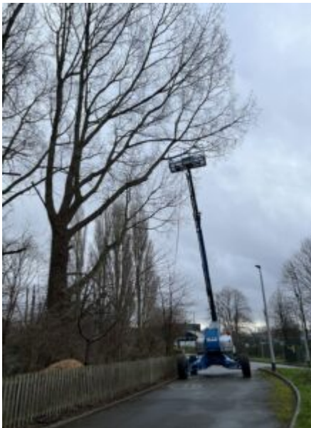
The basket of a mobile elevating work platform (MEWP)
