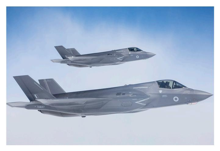
The Lightning, as the aircraft will be known in the UK, is the first to combine radar-evading stealth technology with supersonic speeds and the ability to conduct short take-offs and vertical landings. It will be jointly operated by the Royal Air Force and the Royal Navy and can operate from land and sea, forming a vital part of 'carrier strike', the use of the aircraft from Britain's new Queen Elizabeth Class aircraft carriers.
