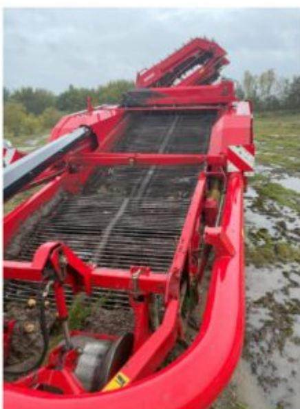
An investigation by the Health and Safety Executive (HSE) found the guard gates to the machine were open and the machine was not isolated. LP Ollier & Son failed to prevent access to dangerous parts of machinery, namely the rotating parts of a potato harvester by means of implementing and following a suitable safe system of work.
