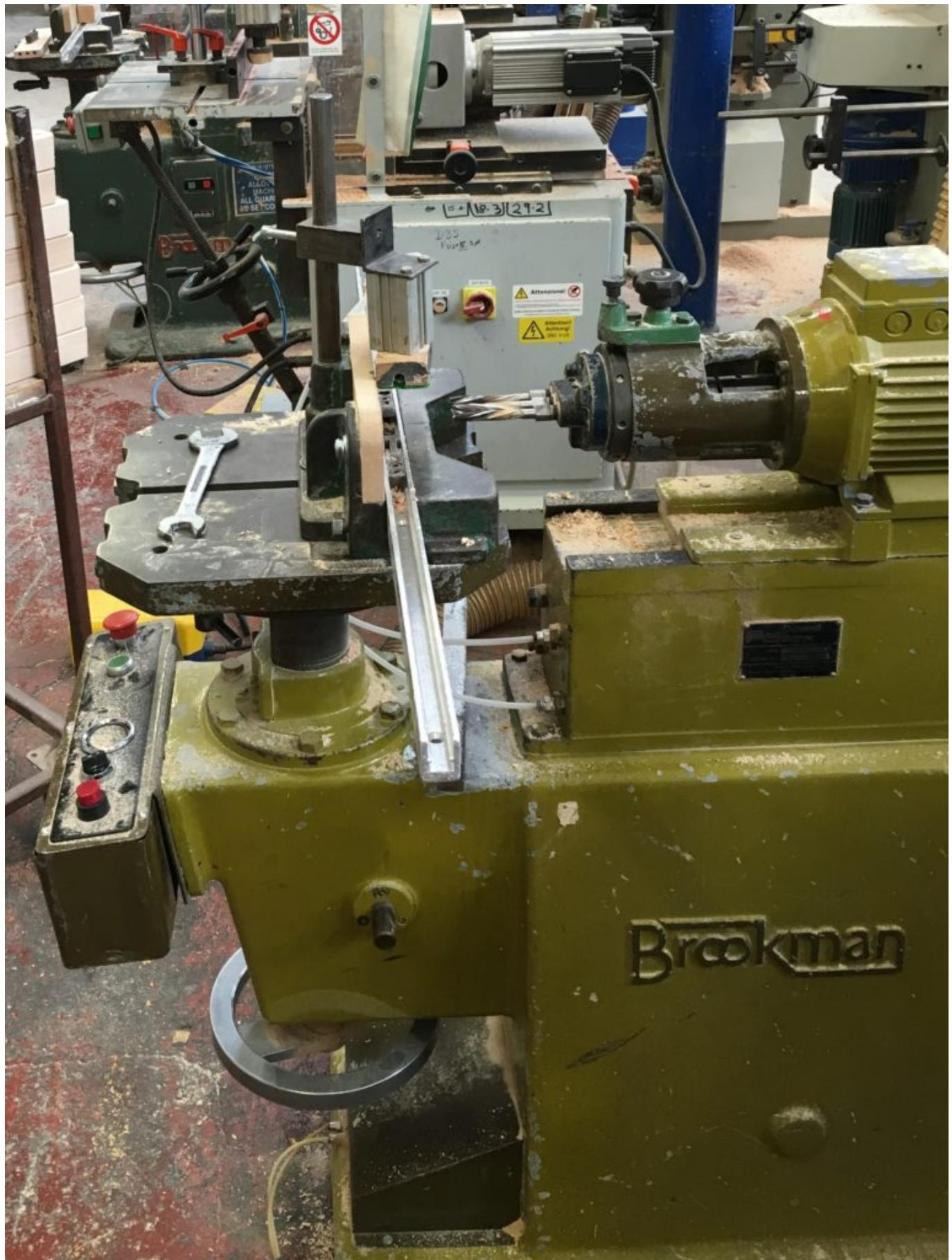
The Health and Safety Executive (HSE) investigation found that it was possible for employees to reach the dangerous parts of the horizontal drilling machine when it was in operation as A and L Furnishings Ltd had failed to provide a suitable guard for the machine.
