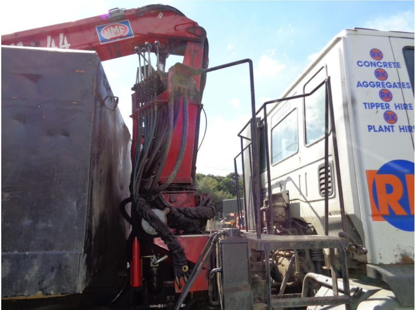
An investigation by the Health and Safety Executive (HSE) found the crane had severe defects, including a disabled safety system, and part of the safety guard around the controls had been cut off, leaving the spike on which his arm was impaled. In addition, the worker had not received appropriate training to operate the lorry loader crane.
