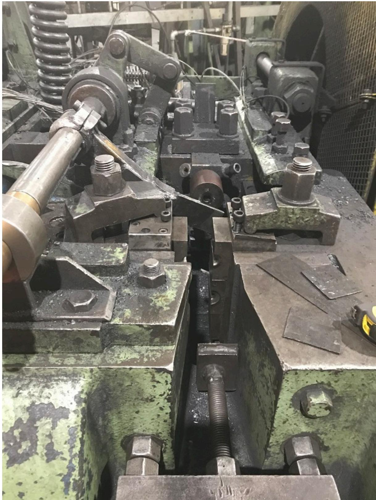
An investigation by the Health and Safety Executive (HSE) found the company had failed to ensure that effective measures were taken to prevent access to the dangerous parts, namely gripping dies and heading tool of the Samuel Platt Upset Forging Press.
