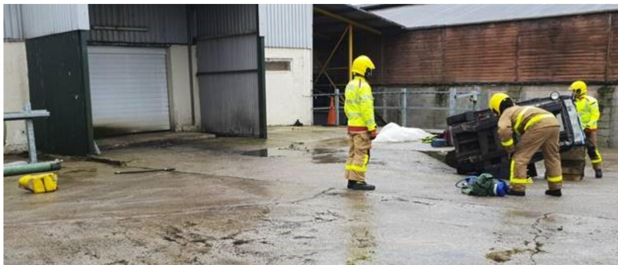
An investigation by the Health and Safety Executive (HSE) found that the areas where FLTs were driven had significant changes in gradient which were not a suitable surface for the type of FLTs in use. The company failed to both identify and control the risk of FLT overturn.
