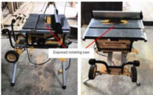
Fig. 2. Dewart DW745-LX Table Saw – shown in the condition that it was used in at the time of the incident - top guard and riving knife removed.
