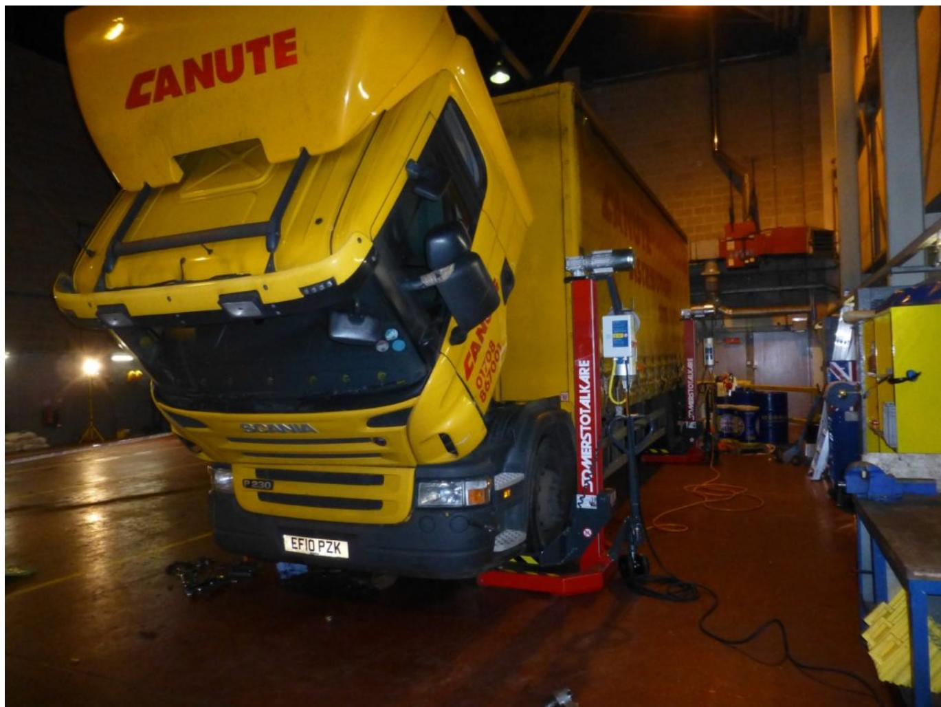
An investigation by the Health and Safety Executive (HSE) found that a cable reel drum jack was used to support the vehicle, which was not an appropriate piece of equipment for the task being undertaken.
