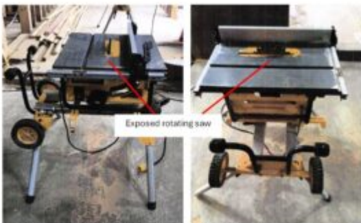
Fig. 2. Dewalt DW745-LX Table Saw – shown in the condition that it was used in at the time of the incident - top guard and riving knife removed.
