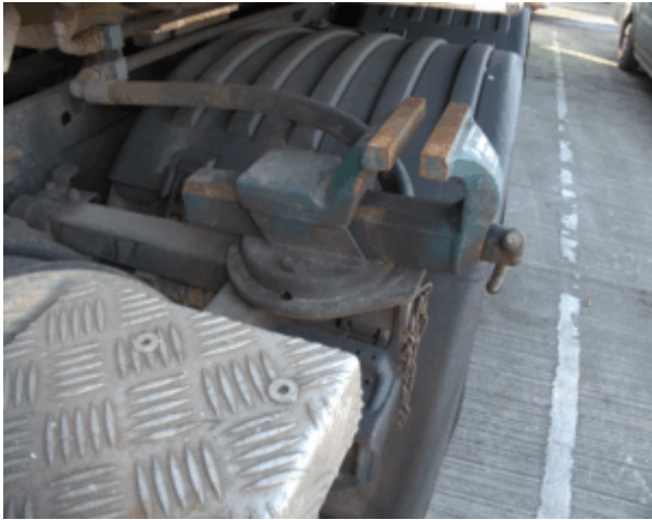
The vice on the vehicle that should secure the hose
