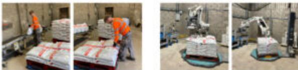
Before: Workers manually palletised 25kg bags from conveyor. This involved constant bending and twisting motions. After: A robotic arm loads bags from conveyor to pallet, which is then wrapped automatically
