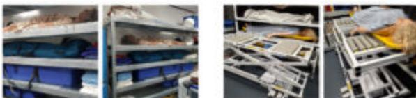
Before: Manikins stored on fixed shelving in a restrictive area, compromising workers' posture when handling. After: Custom roller shelving installed with a height-adjustable roller trolley, eliminating the need to carry the 20kg-40kg manikins to the training area
