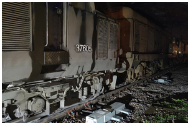
The derailed locomotive
