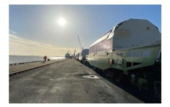
High level waste flasks loaded for transfer to storage site in Germany
