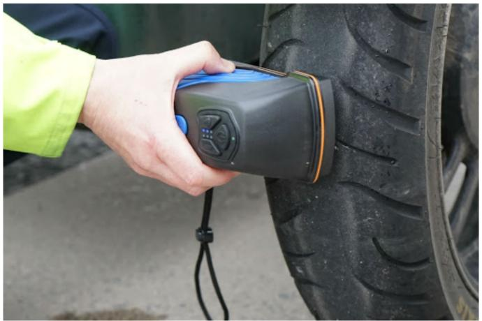
Hi-tech scanners are being used to carry out the free tread and pressure checks
