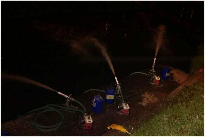
To save the fish, hydrogen peroxide was sprayed to restore the dissolved oxygen levels
