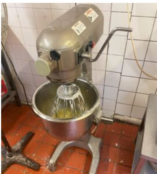
Planetary Mixer missing guard
