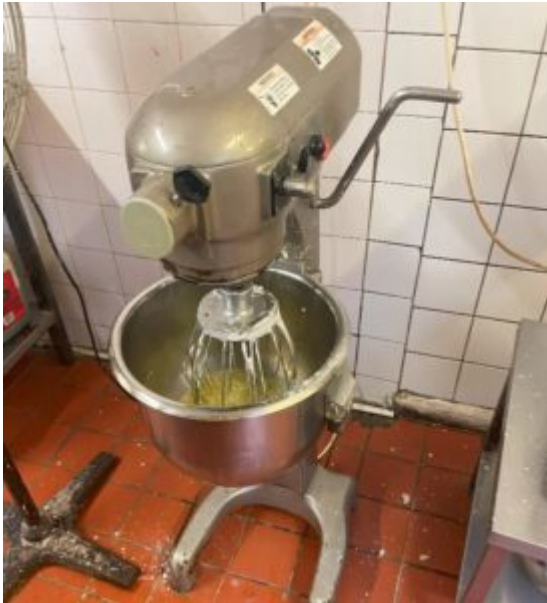
Planetary Mixer missing guard
