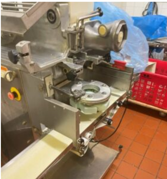
Mochi making machine with missing front guard
