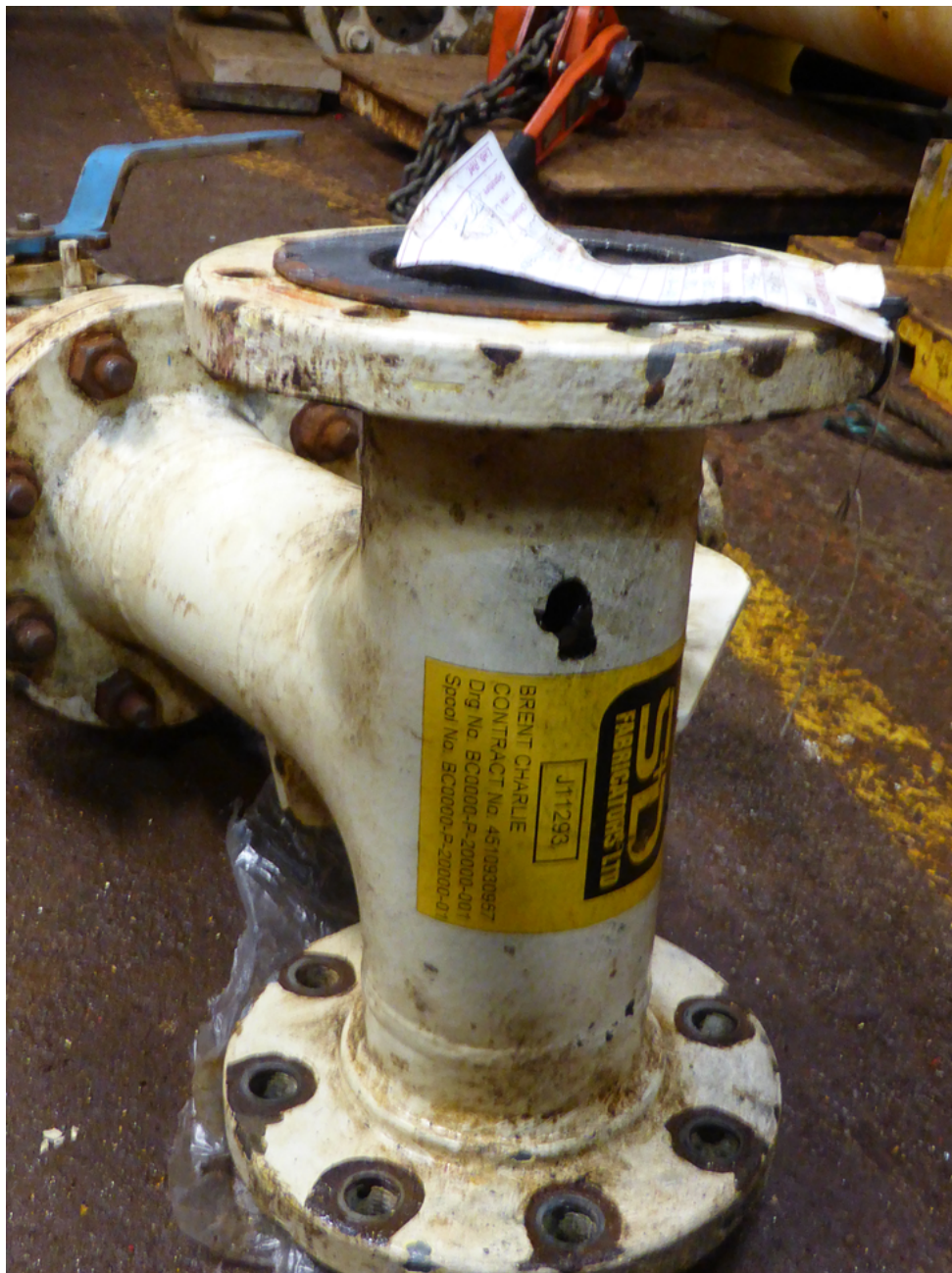
Spool with the corrosion failure identified.
