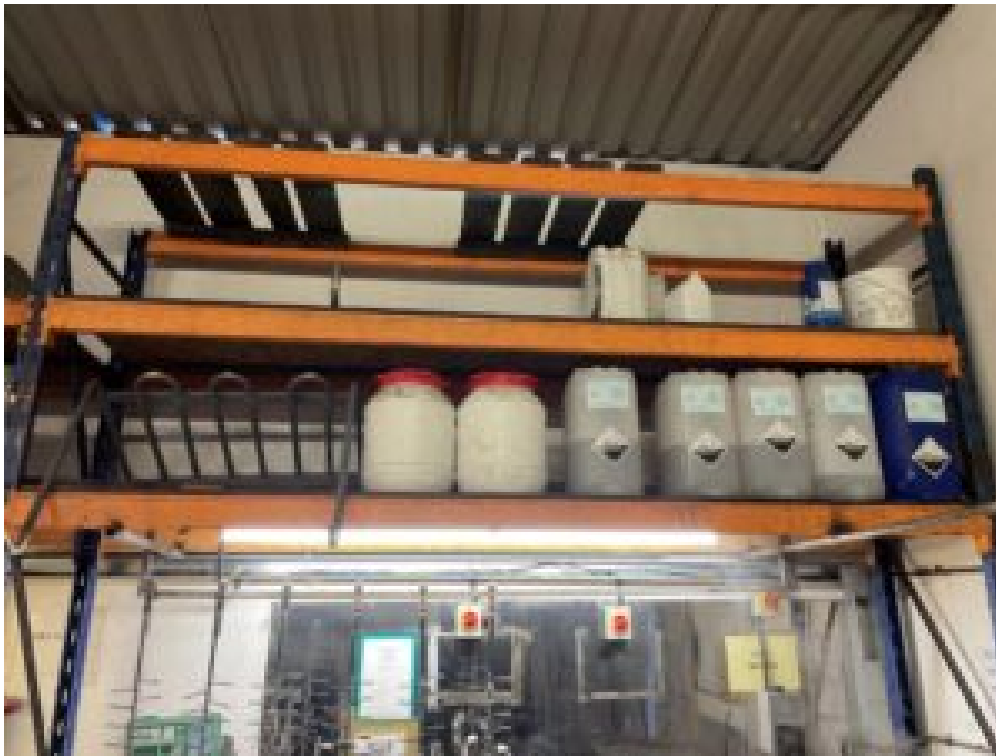
Acids being stored at a high level
