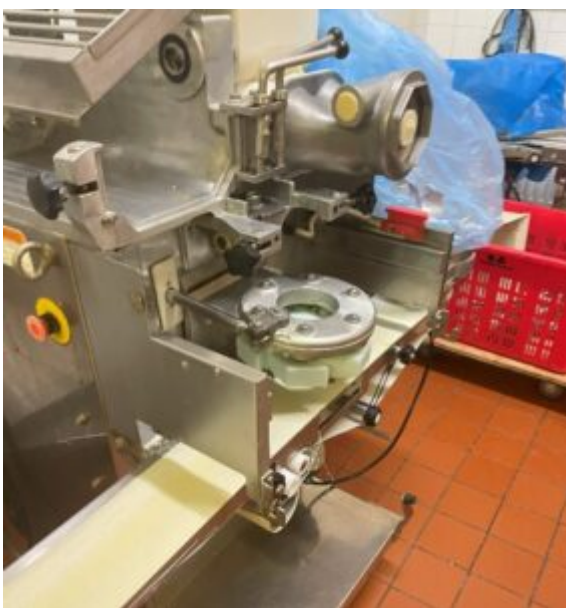
Mochi making machine with missing front guard
