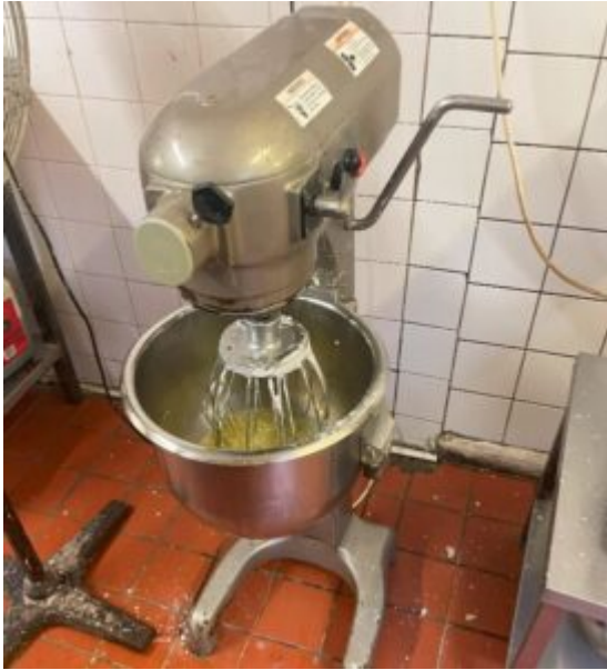
Planetary Mixer missing guard
