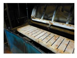
A subsequent investigation by the Health and Safety Executive (HSE) found there was inadequate safeguarding to prevent access between the closing pattern parts of the moulding machine.
