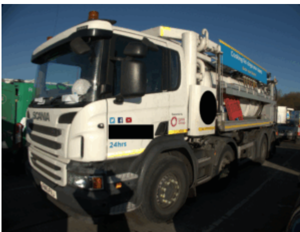
The jetting tanker
