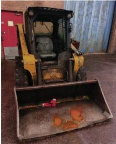
The shovel loader with missing protective door
