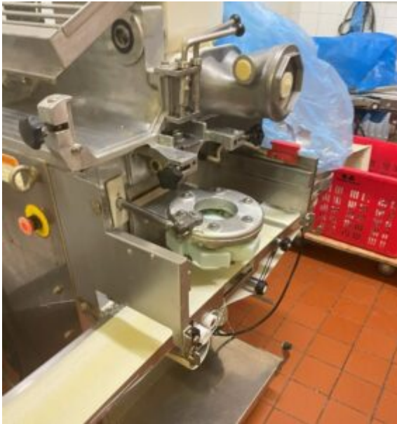
Mochi making machine with missing front guard
