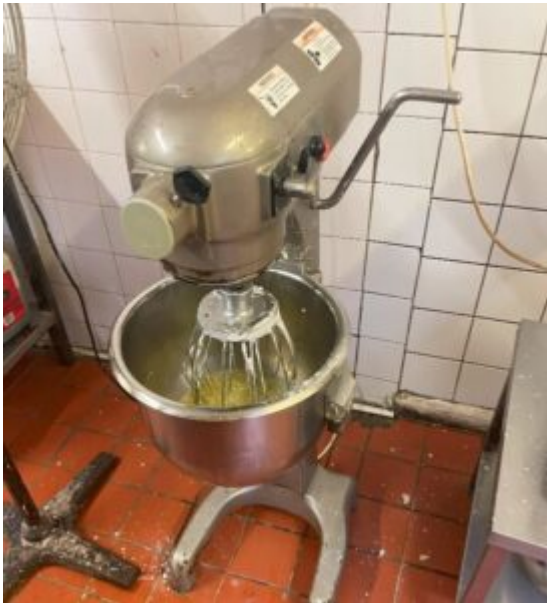
Planetary Mixer missing guard
