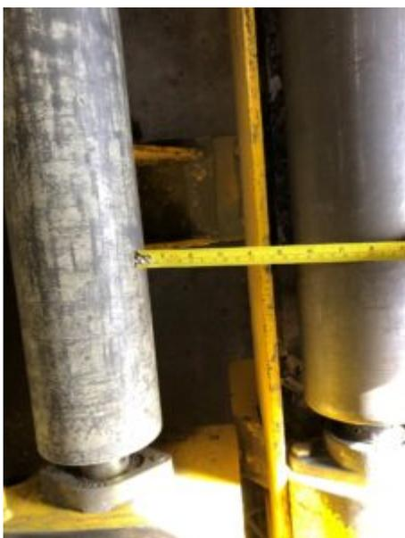
Photo of gap in roller deck pre-accident
