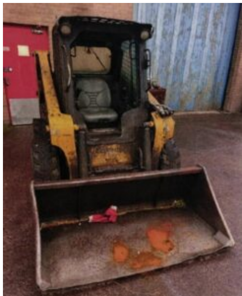
The shovel loader with missing protective door
