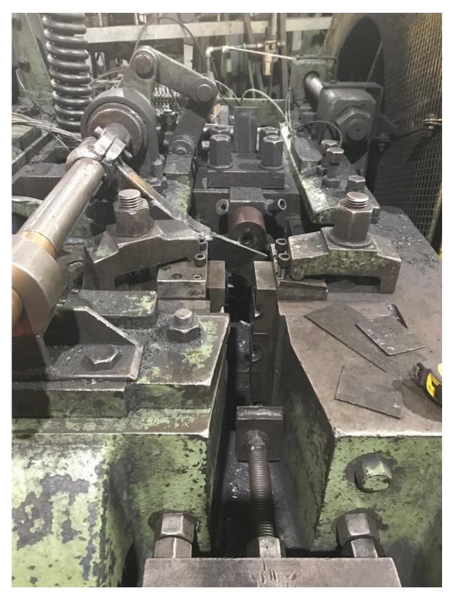
An investigation by the Health and Safety Executive (HSE) found the company had failed to ensure that effective measures were taken to prevent access to the dangerous parts, namely gripping dies and heading tool of the Samuel Platt Upset Forging Press.
