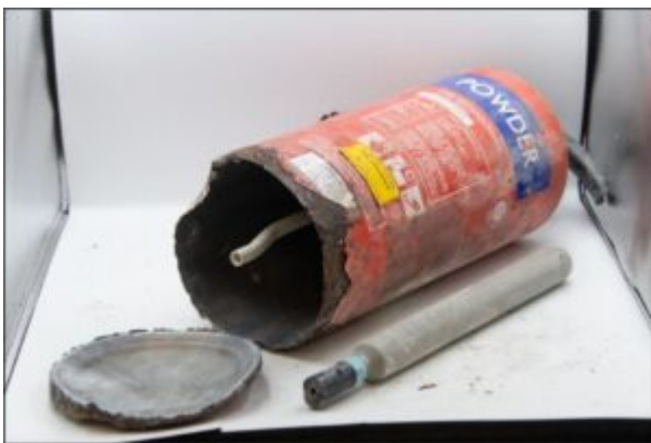
The fire extinguisher that exploded
