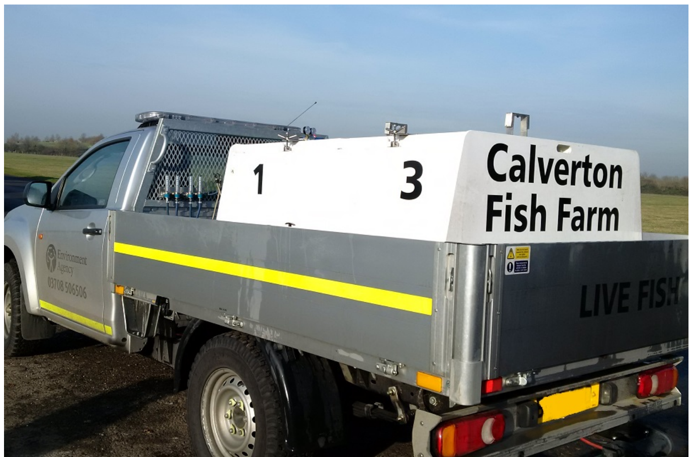
Environment Agency vehicle with oxygenated tanks for transporting live fish.
