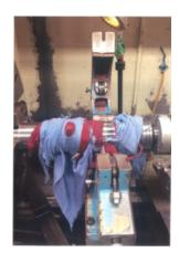
An investigation by the Health and Safety Executive (HSE) found that machinery had interlock devices fitted but they had been by-passed/defeated so it was possible to move guards/doors that should have been interlocked out of the way during set up, to allow access to the rotating chuck and workpiece.
