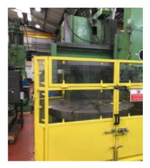
An investigation by the Health and Safety Executive (HSE) into the incident found that the interlocks on the perimeter fencing access doors were not working, and there were no safety checks in place to ensure that the interlocks were in working order.
