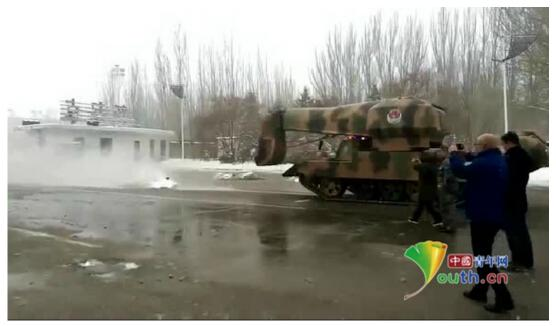
By adapting a jet plane engine to the tank, it can produce high heat to efficiently blow away snow at great distances. [Photo: youth.cn]
