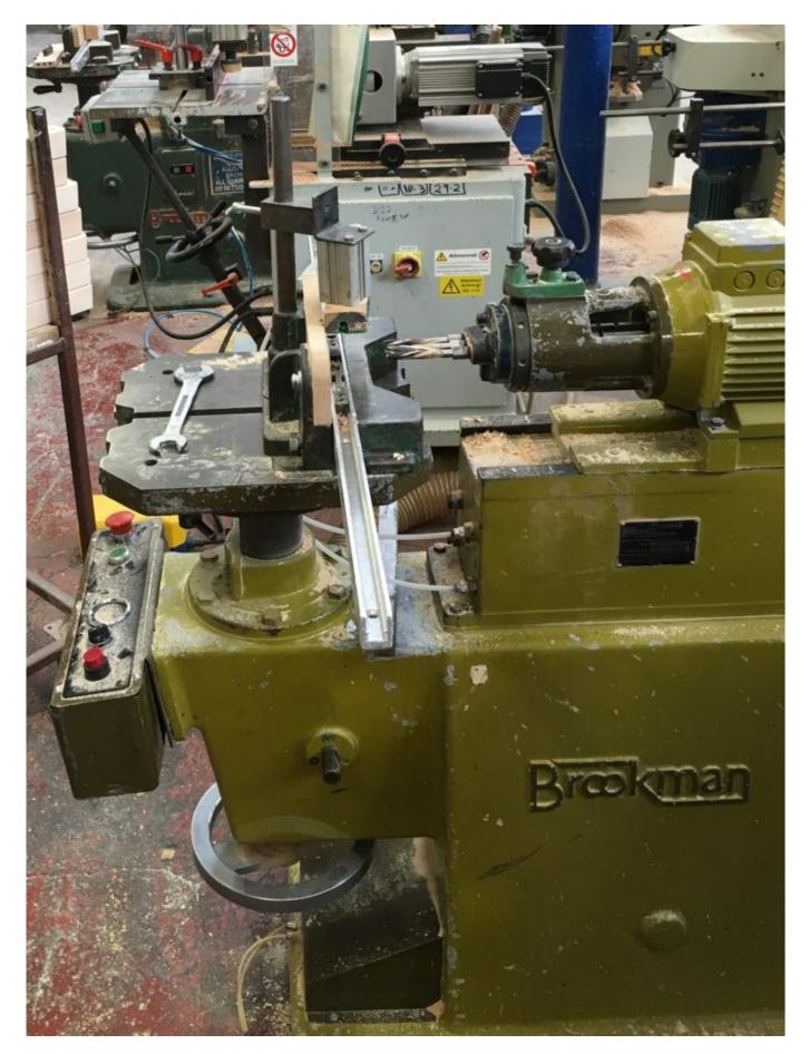
The Health and Safety Executive (HSE) investigation found that it was possible for employees to reach the dangerous parts of the horizontal drilling machine when it was in operation as A and L Furnishings Ltd had failed to provide a suitable guard for the machine. A and L Furnishings Ltd of Leyland, Lancashire pleaded guilty to breaching Regulation 11(1) of the Provision and Use of Work Equipment Regulations 1998 and has been fined of £14,000 and ordered to pay costs of £5500.85.
