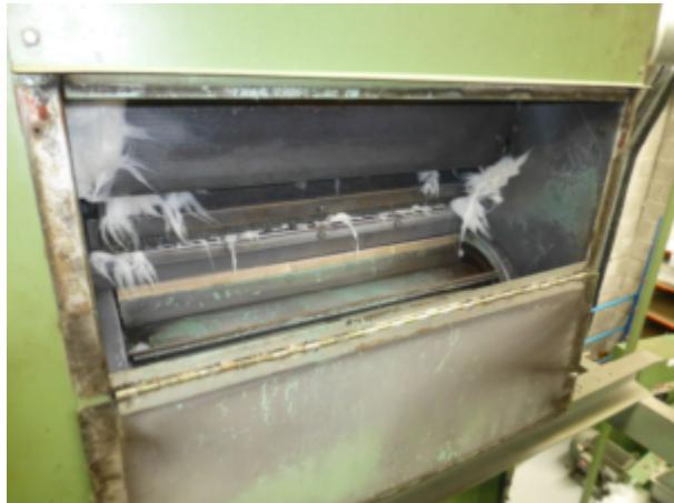
The woman's hand was drawn into the machine after it became blocked with fibres, Image: HSE
