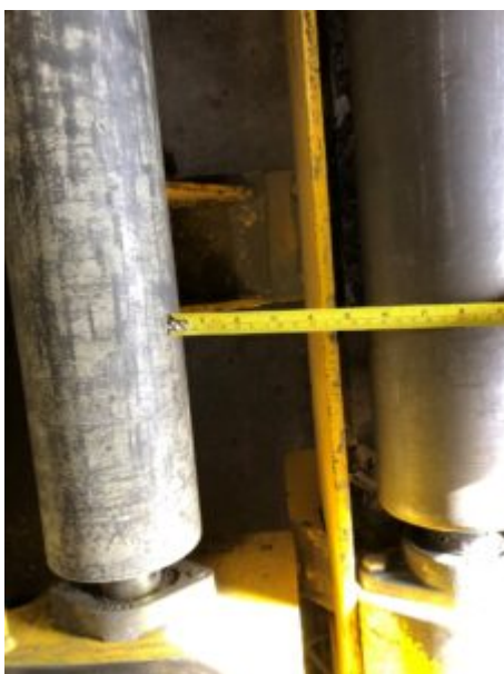
Photo of gap in roller deck pre-accident
