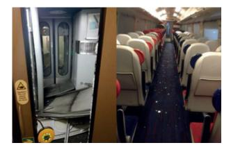
Damage to the vestibule end and debris in the saloon (left image courtesy of CrossCountry, right image courtesy of Bombardier Transportation UK).
